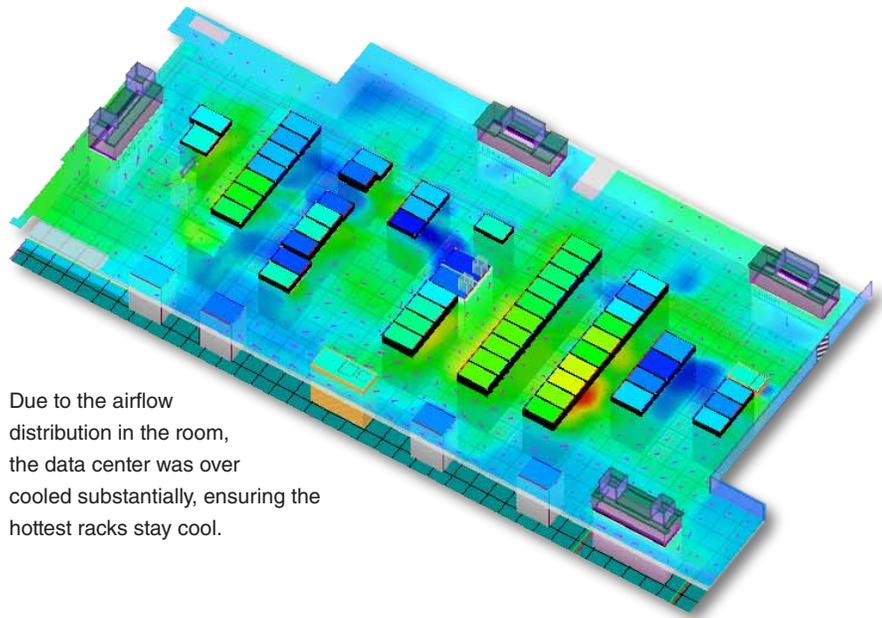
Due to the airflow distribution in the room, the data center was over cooled substantially, ensuring the hottest racks stay cool.
