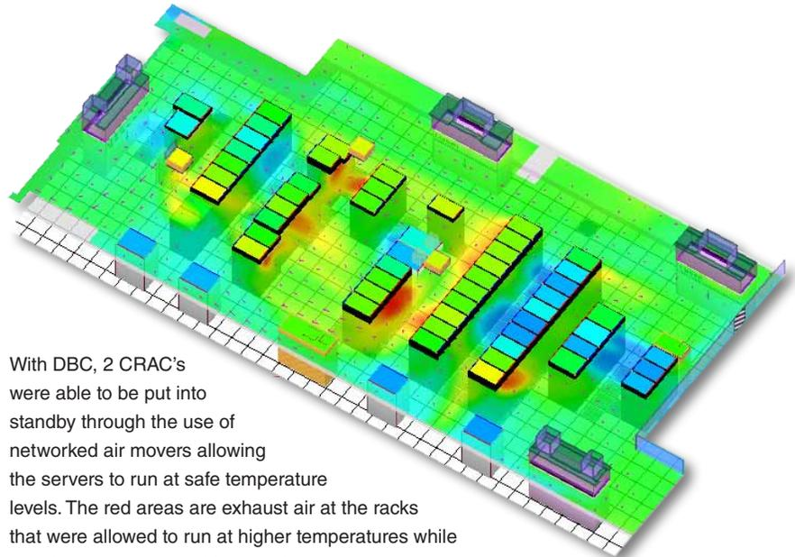
With DBC, 2 CRAC's were able to be put into standby through the use of networked air movers allowing the servers to run at safe temperature levels. The red areas are exhaust air at the racks that were allowed to run at higher temperatures while maintaining proper inlet temperatures.
